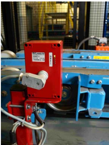
P3313054: On the back of the read stations, operating states such as voltage supply, warning signal, pre-clock signal, clock signal, and info signal are displayed via LED.
