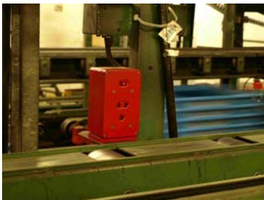
P3313087, P3313089, P3313090: Three polarization filter Light Beam Devices and above an additional light scanner are contained in the compact housing of the new read stations.
