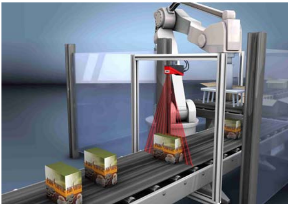
Figure 6. In this grabber control, the 3D data of the parts on the moving conveyor can be captured with the LPS sensor.
