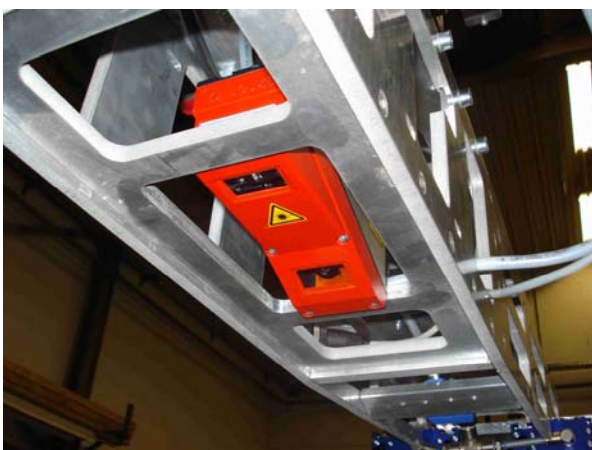
Figure 4. The LPS light-section sensors from Leuze electronic are characterized by their compact construction.
