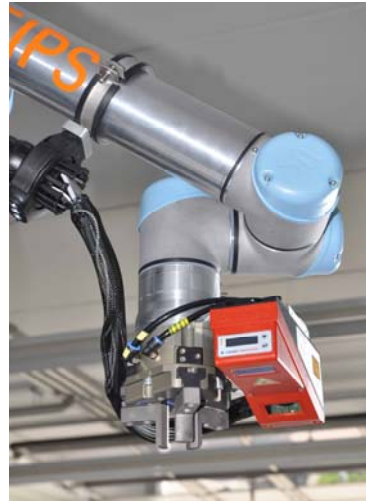
Figure 2. Robot with light-section sensor
