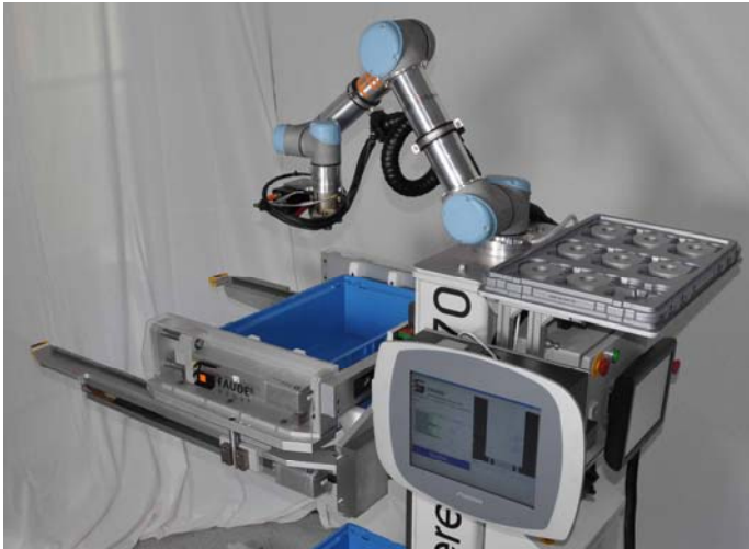
Figure 1. Using a lightweight robot to precisely set down parts
