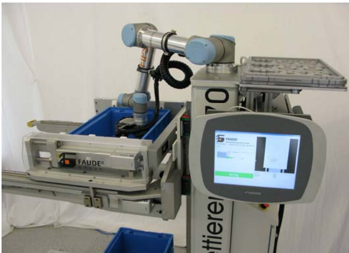
Figure 3. The working radius is up to 850 mm, repeatability \pm 0.1 mm
