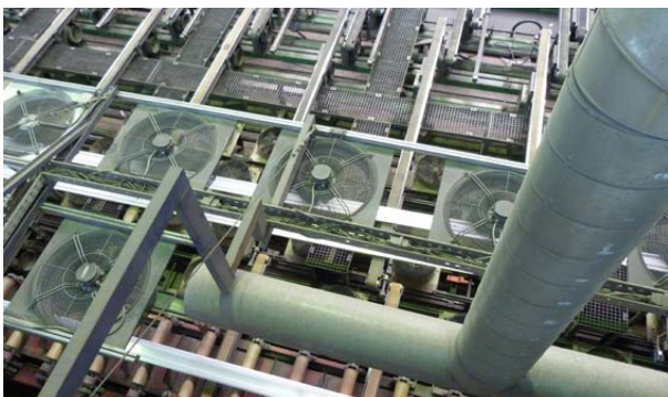
Figures 4a and 4b. Four rows of 45 fans cool the pressed profiles.
