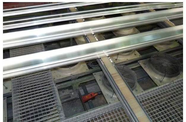
Figures 3a and 3b. The aluminum profiles are transported in run-out lengths of up to 60 meters over a refrigerated table to the cold saw roller table.
