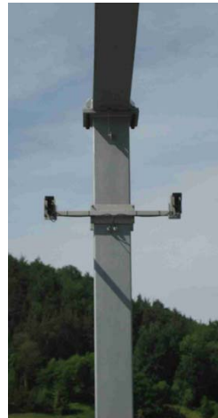
Figures 2a/b. The robustly built LS 96 One-way Light Beam Devices from Leuze electronic also fulfill the requirements on the highway for every type of weather. Redundantly installed, these One-way Light Beam Devices also guarantee maximal functional reliability outdoors.
