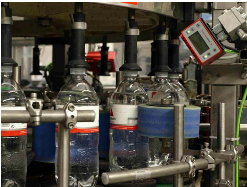
Figure 2. Compact and robust – the LSI 412i smart cameras can be integrated easily into beverage filling systems.
