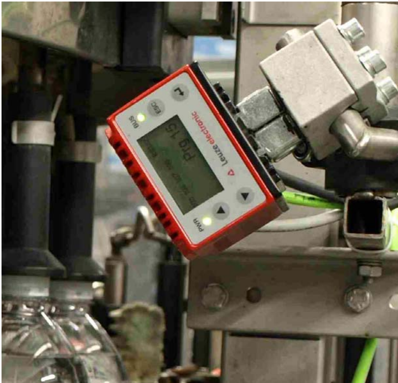
Figure 3. Illumination, image processing, image and program memory, display, result display and interfaces – everything is contained in compact industrial-grade metal housing, which can be very easily mounted due to the fastening concept.
