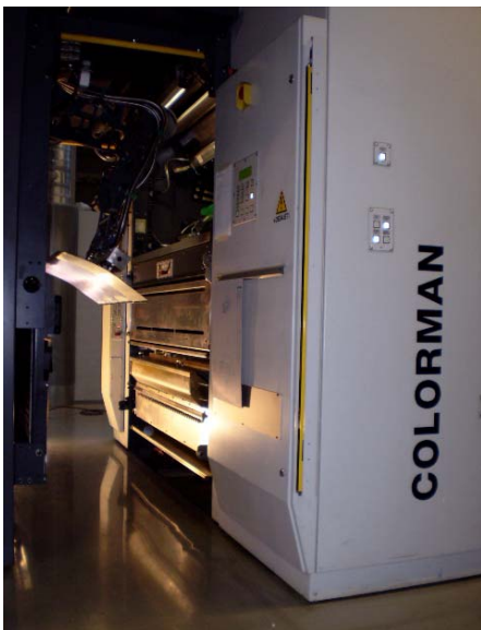
Pict. 1: Safety Light Curtains as access guarding with a fully automated system for loading printing plates
