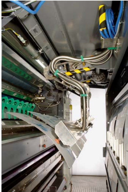
Pict. 6: Loading the printing plates into the cylinder (left) with the APL system
