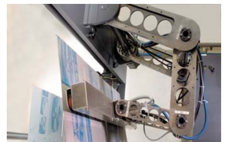
Pict. 2: Mechanically stable Automatic Plate Loading (APL) system handling printing plates
