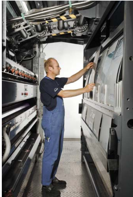
Pict. 4: Manual loading the printing plates before starting the APL system
