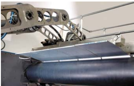
Pict. 3: Winding the printing plates with the APL system
