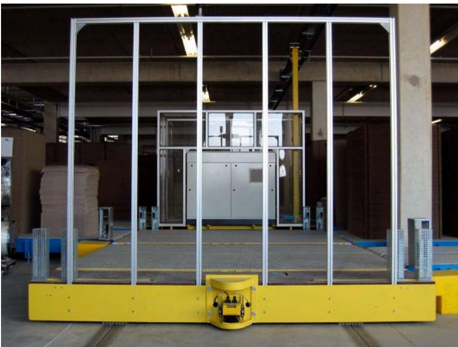
Pict 1: Transfer trolley with mounted Safety Laser Scanners for travel path guarding
